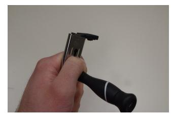
Carefully pull the pick out of the spring coils. Be sure to hold a hand over the end of the magazine so that the spring can't go flying. Completely remove the spring from the magazine.
