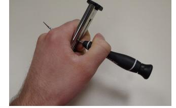
2. Slide the base pad off the end of the magazine and set it aside.
