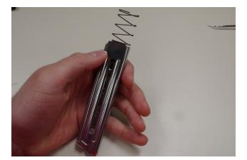
Slide the base pad back onto the end of the magazine. Remove the pick. Slide the follower button up and down a few times to ensure that everything moves the way it's supposed to and that the spring is seated on the base pad correctly.
