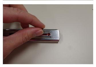
Re-insert the spring, pushing the follower all the way to the top of the magazine. Then insert the pick into the coils of the spring and pull towards the follower until the entire spring is inside the magazine. Hold the pick in place there.
